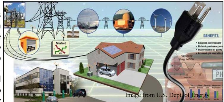
AMI is a network that allows two-way communication between smart meters and a utility company's electrical system. AMI enables the company to collect usage data, by customer, on an hourly basis so consumers can track and alter their energy use as a way to minimize their bills.
